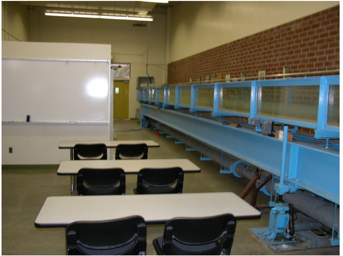
Photo 3.8: 50ft. Hydraulic Channel (Hydraulics Laboratory)
