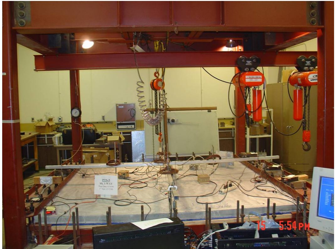
Photo 3.2: 3-D Structural Test Frame (Structures Laboratory)
