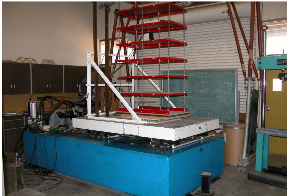
Photo3.4: Seismic Shake Table (Structures Laboratory)
