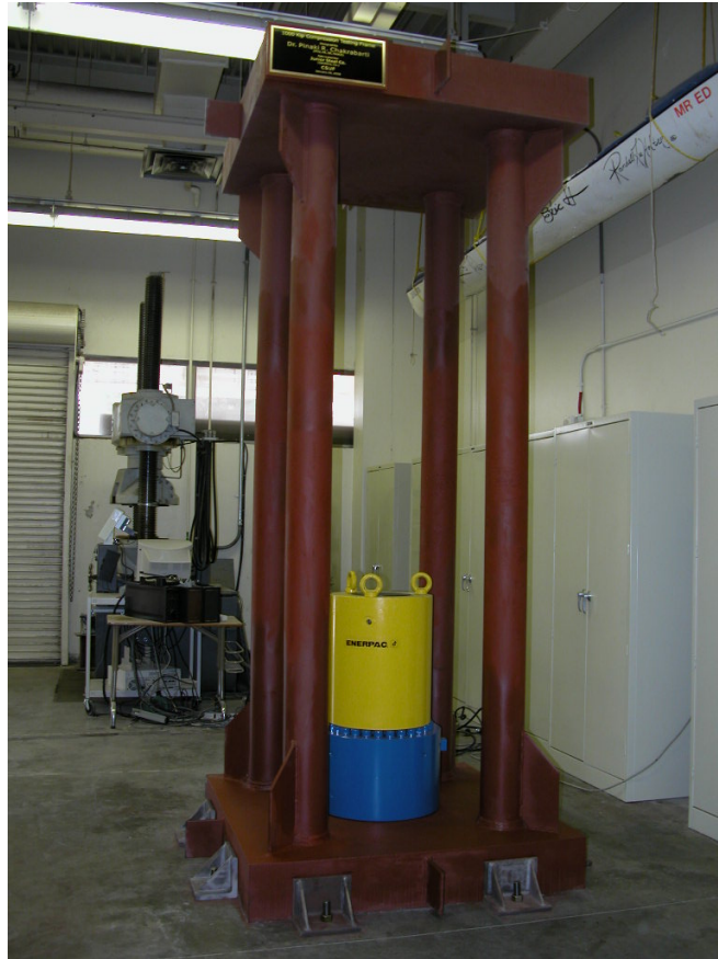
Photo 3.3: 1000-kips Compression Test Frame and 200k Universal Testing Machine Beyond (Structures Laboratory)
