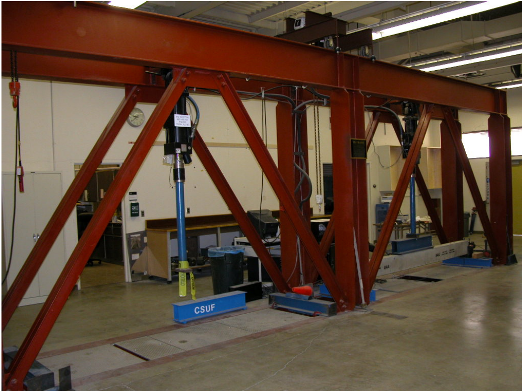
Photo 3.1: 2-D Structural Test Frame (Structures Laboratory)
