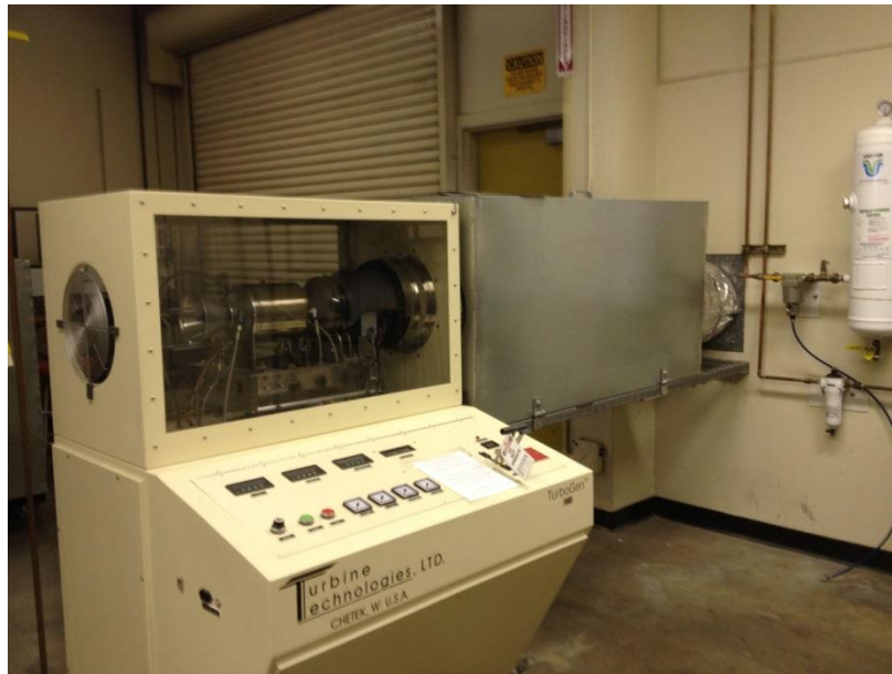
Figure 7.12 Turboggen Gas Turbine Electrical Generation System
