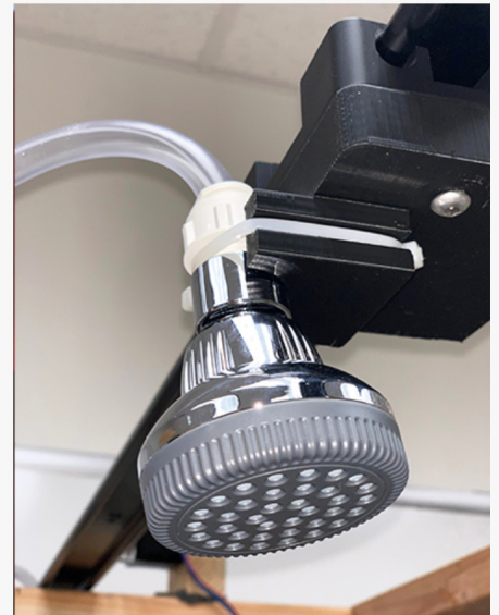
Computer engineering students designed this showerhead on a motorized track to enable the shower to operate by using voice recognition.
