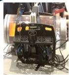
**Autonomous Submarine:** Underwater vehicle capable of following paths and avoiding obstacles (being developed to enter into the RoboSub Competition).
