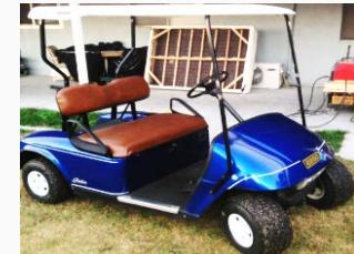
Tuffy Cart follows specified routes using GPS and Mission Planner software to assist anyone in need of easier transportation around campus.
