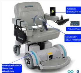
Brain-computer interface (BCI) based system to control an electric wheelchair thoughts and facial expressions.
