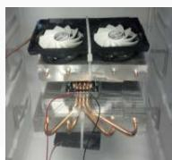
Design and implementation of a solar Powered enclosure which utilizes the Peltier effect to provide refrigeration and heating methods.
