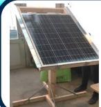
**Solar-Tracking & Self-Cleaning System for Solar Panels:** System with dual-axis motion solar tracker and self-cleaning mechanism improves the amount of harvested energy.
