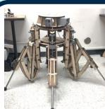
**MiniDex:** An omnidirectional 6-legged symbiotic robot designed for applications in assisting in anti-fatigue, strenuous, and repetitive activities.
