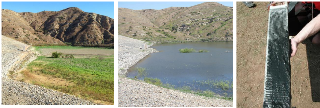
Left, Villa Park Dam in November 2008; Middle, Villa Park Dam in April 2009; Right, an example of a “Peeper”, which is used to obtain cm-scale samples of sediment-pore water with depth
